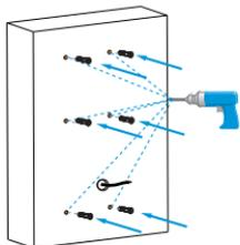
Use a hand drill with 5 mm diameter bit to make the holes in marked positions. And then insert the plastic wall anchors into the holes.
