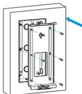
Use six M4x10 screws to fix the flush-mounting bracket on the embedded box.
