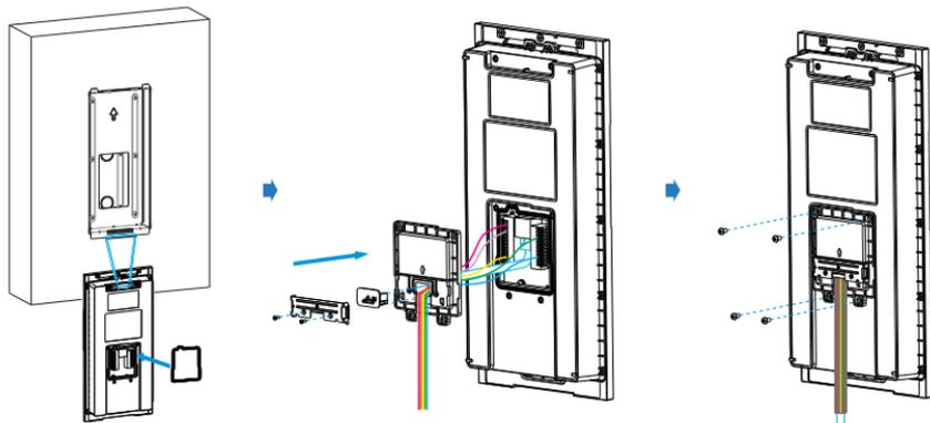
For convenient wiring, hang R27X on the wall-mounting box/flush-mounting bracket with rope. Then insert the silicon rubber sealing ring into the groove.
