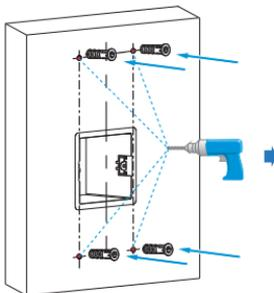
Take off the box and drill the four marked holes with a depth of 25 mm using 5 mm drill bit hand drill before inserting the plastic wall anchors into the drilled holes.
