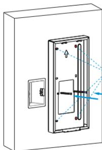
Fix the wall-mounting box on to the embedded box (86) with two M4x30 screws, mark the positions of the four holes of the wall-mounting box at the hole center.
