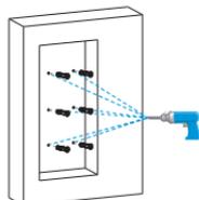
Take off the box and drill the holes on the marked positions with a depth of 25 mm using 5 mm drill bit hand drill before inserting the plastic anchors in to the drilled holes.
