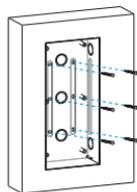
Break off the round knock-out wiring holes and lead the wires through the corresponding hole in to the flush-mounting box, then press the flush-mounting box in to the square hole until the edges of which align to the wall. Then fix the box using the four ST4x20 screws.
