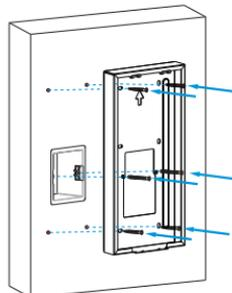
Fix the wall-mounting box with four ST4x20 screws and two M4x30 screws.
