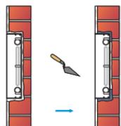
Use cement or non-corrosive structural adhesives to fill the gap between the wall and flush-mounting box. Wait the adhesive material desiccation, go to the next step.
