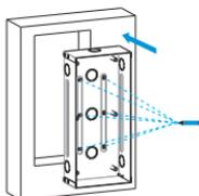
Insert the flush-mounting box in to the hole and mark the the positions of the six holes of the flush-mounting box on the wall.
