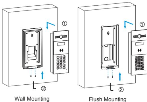
1. Place the device into the wall-mounting box/flush-mounting bracket until the edges of which align to the wall. Then pull the device downward and ensure the groove of it hooks to the lock catches of the back box.
