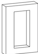
Cut out a square hole with the dimension height\*width\*depth = 264\*122\*61 mm.
