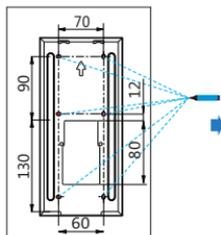
According to the position of the wire on the wall, put the wall-mounting box closely on to the wall and mark the six positioning holes, while making sure that relative positions between wall-mounting box and wiring hole are correct.
